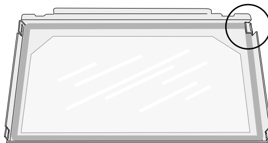
Figure 54. Bend the retainer tabs back enough to release the glass panel.
