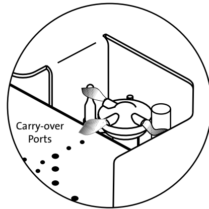
Figure 37a. Proper pilot flame appearance relative to burner carry-over porting.
