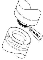
RE-INSTALL THE TOP PLATE BEFORE CONNECTING VENT TO THE STOVE.
