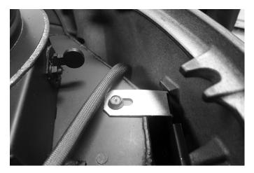
Figure 16.2. Remove the firebox-to-side plate bolt.
