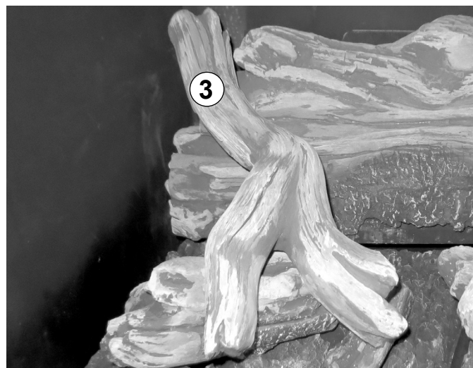
Figure 7.29. Engage holes in the underside of #3 Left Upper Log with the pegs on Logs #1 and indents on log #2, resting on log #2.
