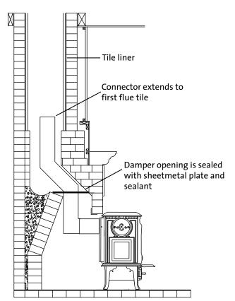
The inside area of the flue liner must not be less than the area of the stove's flue exit, and cannot be more than three times greater than the cross sectional area of the stove's flue exit. If the chimney liner is too large to accommodate the stove, an approved relining system must be installed to resize the flue. A new sheet metal damper block-off plate must be installed around the connector pipe at the damper frame and sealed with the proper sealant (usually high-temp silicone).
