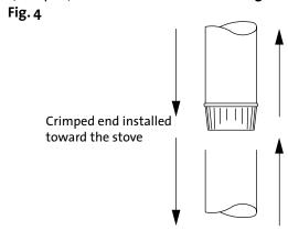
This prevents any amount of condensed or liquid creosote from running down the outside of the pipe or the stove top. All joints must be secured with three sheet metal screws to ensure that the sections do not separate.
