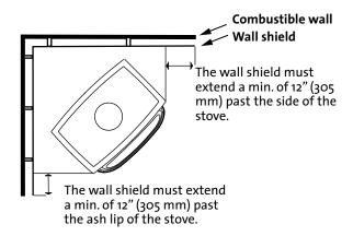
Must be 1" off the wall and 1" off the floor. With standard legs, the shield must be 40" high. With optional short legs, the shield must be 38" high. Both shields must extend and join in the corner.
