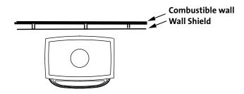
Must be 30" wide and centred behind the stove. Must be 1" off the wall and 1" off the floor. With standard legs, the shield must be 32" high. With optional short legs, the shield must be 30" high.
