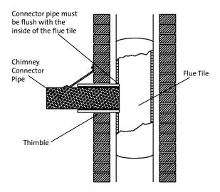
Make sure the connector pipe or thimble sleeve does not protrude into the flue liner, thereby restricting the area the smoke has to flow through. This bottle-neck will have a negative affect on the chimney system.
