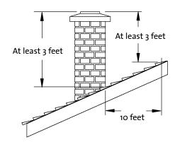
Chimneys shorter than 15 feet may not provide adequate draft. This could result is smoke spilling into the room from the stove when loading the stove, or when the door is open. In addition, inadequate draft can cause back puffing, which is a build up of gases inside the firebox.
